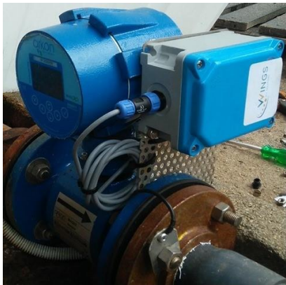
Figure 1. WINGS Nb-IoT based device for enabling smart water management, consumption monitoring/predictions and fault management
