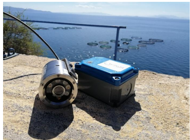
Figure 2. Camera to be installed underwater, for monitoring the production, and to transmit through cabling and 4G/5G.
