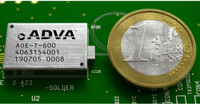
IC-TROSA type 1 SMT package (reflow-soldering capable)
